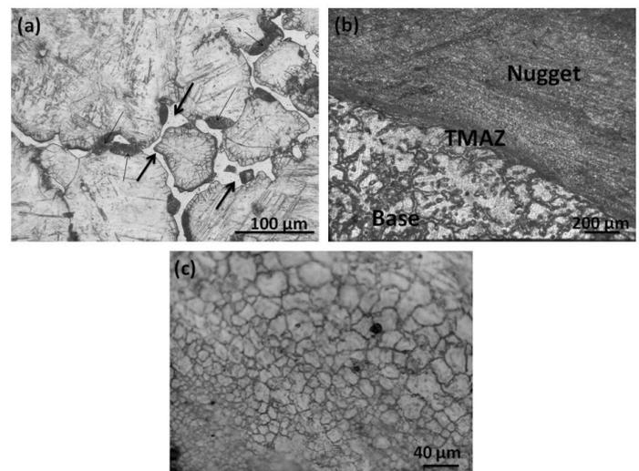
Figure 2 Optical microscope images of the samples: a) unprocessed AZ91, b) FSPed AZ91 and c) magnified image obtained at the nugget zone of FSPed AZ91
