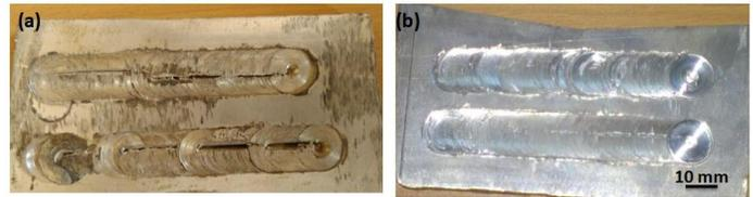
Figure 1 Photographs of FSPed AZ31 sheets: (a) 1400 rpm tool rotational speed and 25 mm/ min tool feed and (b) 1400 rpm tool rotational speed and 20 mm/ min tool feed.
