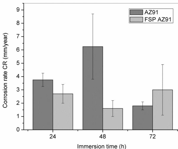
Figure 3 corrosion rates of the samples calculated from the immersion tests.
