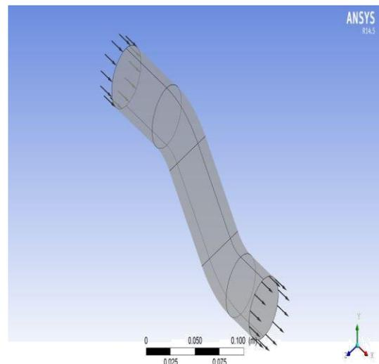
Fig. 3- Boundary conditions in CFX
