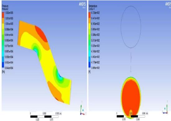
Fig. 4 - Variation of temperature and pressure at outlet
