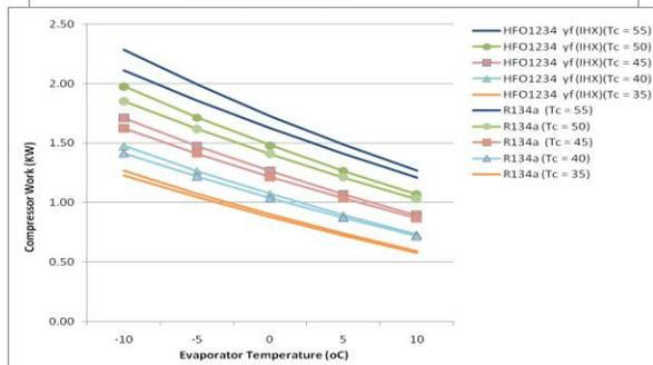
Fig.7 – Theoretical Compressor work Vs. Evaporator Temperature (At varying Condenser Temp) (With & without Heat Exchanger)
