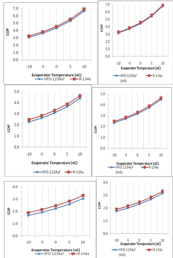
Fig.5 – COP Vs. Evaporator Temperature at Condensation Temp 35 °C A) Without IHX , B) With IHX , at Condensation Temp 45 °C C) Without IHX & D) With IHX & at Condensation Temp 55 °C E) Without IHX & F) With IHX
