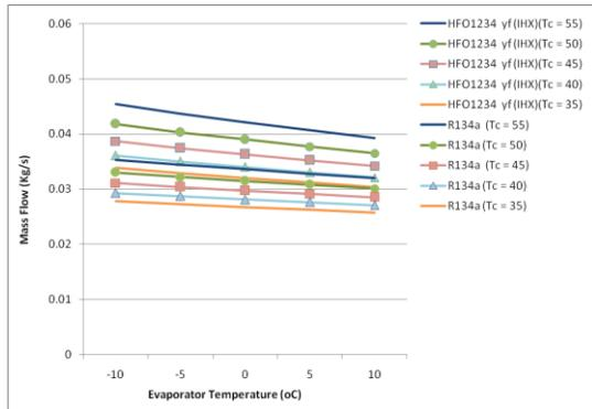
Fig. 6– Theoretical Mass flow rate Vs. Evaporator Temperature (At varying Condenser Temp) (With & without Heat Exchanger)
