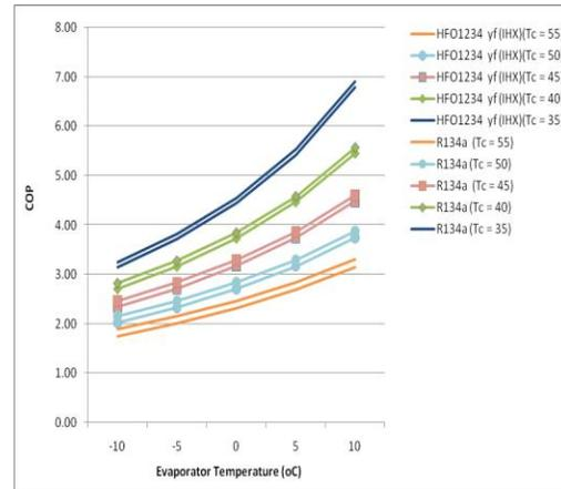
Fig.8 – Theoretical COP Vs. Evaporator Temperature (At varying Condenser Temp) (With & without Heat Exchanger)
