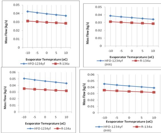
Fig.3 – Mass flow rate Vs. Evaporator Temperature at Condensation Temp 35 °C A) Without IHX , B) With IHX , at Condensation Temp 45 °C C) Without IHX & D) With IHX & at Condensation Temp 55 °C E) Without IHX & F) With
