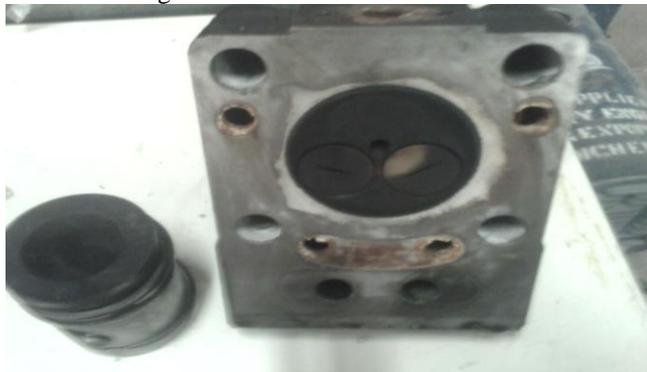
**Figure 1: Zirconium Oxide coated piston and head**
