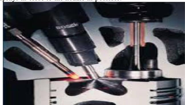
**Figure 2. Sectional view of piston cylinder assembly showing the glow plug and fuel injector arrangements.**
