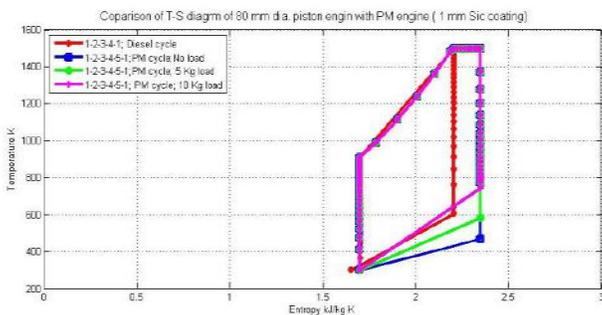
Figure 5. Comparative T-S diagrams for 80mm dai. Piston engine
