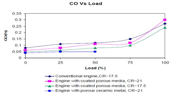
Figure 7. Comparison of carbon monoxide emission
