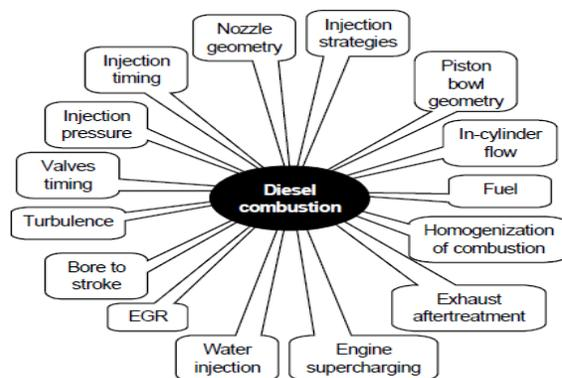
Figure 1. Available Technology for DI diesel Engine.
