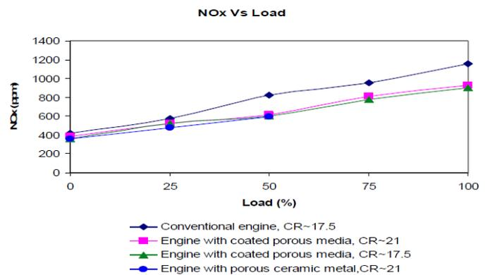
Figure 8. Comparison of nitrogen oxide emission
