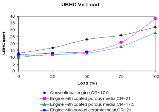
Figure 6. Comparison of hydrocarbon emission
