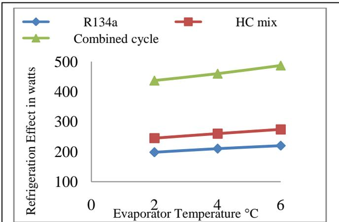
Figure 5: Variation of refrigeration effect with evaporator
