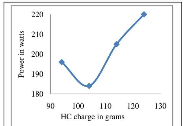
Figure 3: Optimization of HC mix charge
