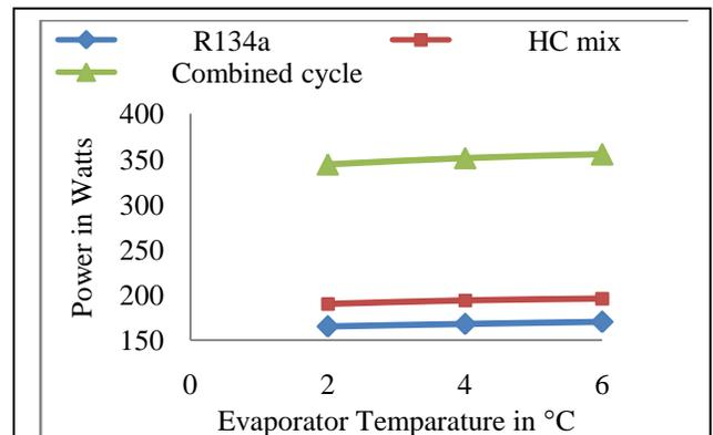
Figure 4: Variation of Power with evaporator temperature
