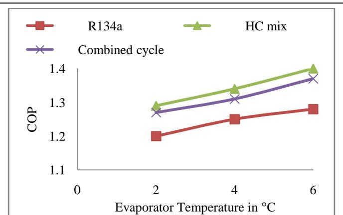
Figure 6: Variation of COP with evaporator temperature
