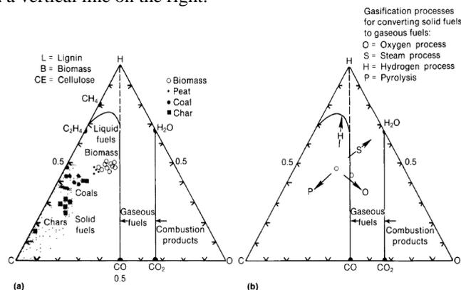
**Figure 1: Relative proportions of C,H,O in solid, liquid and gaseous fuels.**
