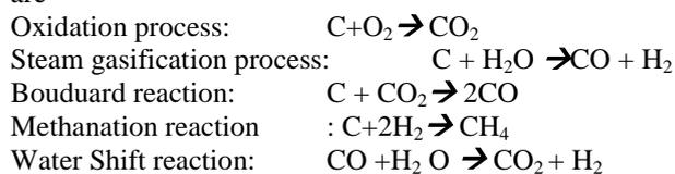
Out of these only four reactions are independent reactions, which are chosen as oxidation, steam gasification, bouduard reaction, and the methanation reaction. The water gas shift reaction can be considered as the subtraction of the steam gasification and bouduard reactions. Oxidation reaction is typically assumed to be very fast and goes to completion (Von Fredersdorff and Elliott, 1963) and three reactions namely bouduard reaction, steam gasification and methanation are in equilibrium.
