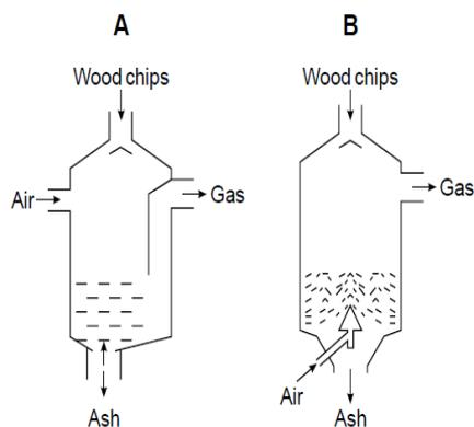
**Figure 2: Schematic of updraft and downdraft gasifiers**
