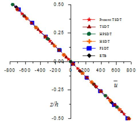
Fig. 3. Variation of axial displacement ( $\bar{u}$ ) through the thickness of beam at ( $x = 0.75L$ ,  $z$ ) for aspect ratio 4 and 10.
