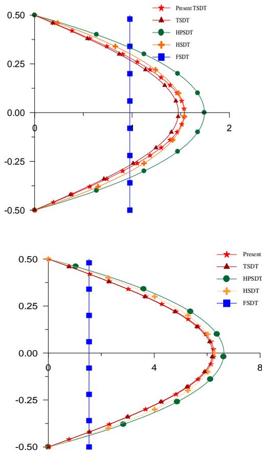
Fig. 5. Variation of transverse shear stress ( $\bar{\tau}_{zx}$ ) through the thickness of cantilever beam at ( $x=0.01L, z$ ) obtain using constitutive relation for aspect ratio 4 and 10.
