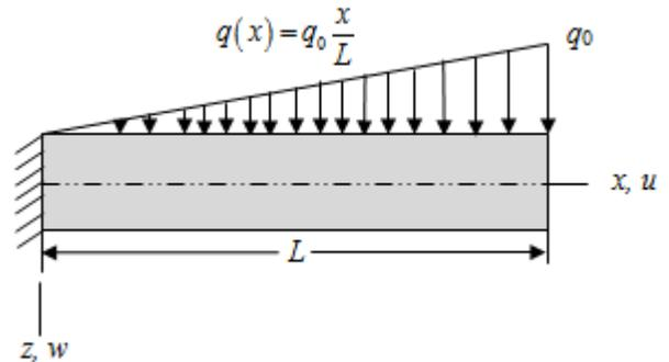
Fig. 2. Cantilever beam with uniformly varying load
