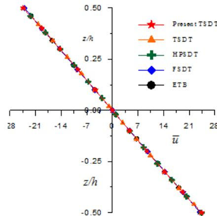
Fig. 2. Variation of axial displacement ( $\bar{u}$ ) through the thickness of beam at  $(x = 0.75L, z)$  for aspect ratio 4 and 10.
