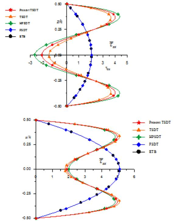
Fig. 6. Variation of transverse shear stress ( $\bar{\tau}_{zx}$ ) through the thickness at ( $x=0.01L, z$ ) obtain using EE for  $S=4$  and  $10$ .
