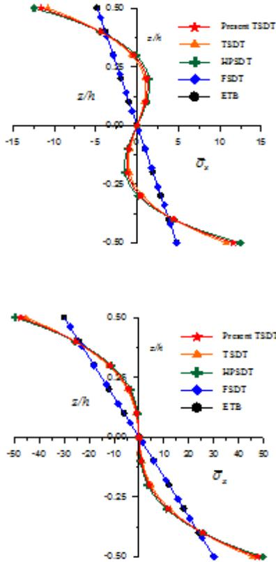
Fig. 3. Variation of axial stress ( $\bar{\sigma}_x$ ) through the thickness at ( $x=0, z$ ) for  $S=4$  and  $10$ .
