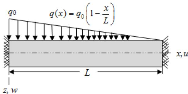
Fig. 1 Fixed beam with varying load
