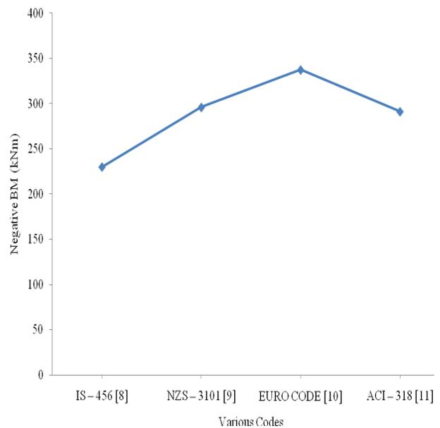
**Fig. 4:** Variation of Negative Bending Moment by various codes and with MATLAB
