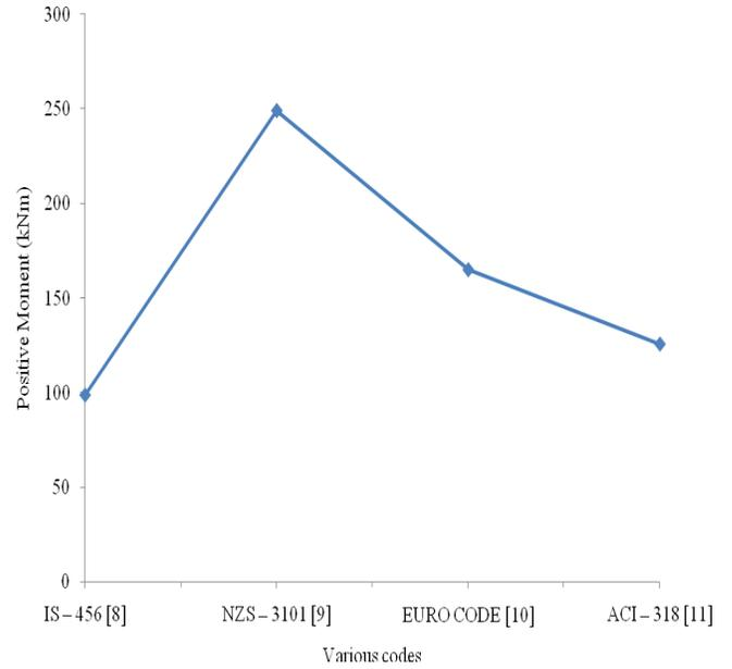
**Fig. 3:** Variation of Positive Bending Moment by various codes and with MATLAB
