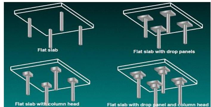
Fig. 2: Different Profile of Flat Slab
