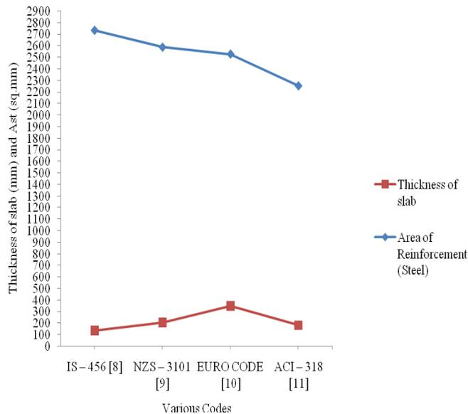
**Fig. 5:** Variation of Thickness of Slab (mm) and Area of reinforcement (mm<sup>2</sup>) by various codes and with MATLAB
