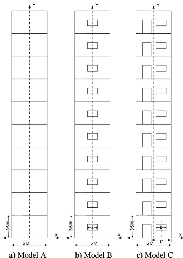
**Figure 2. Shear Wall Models**
