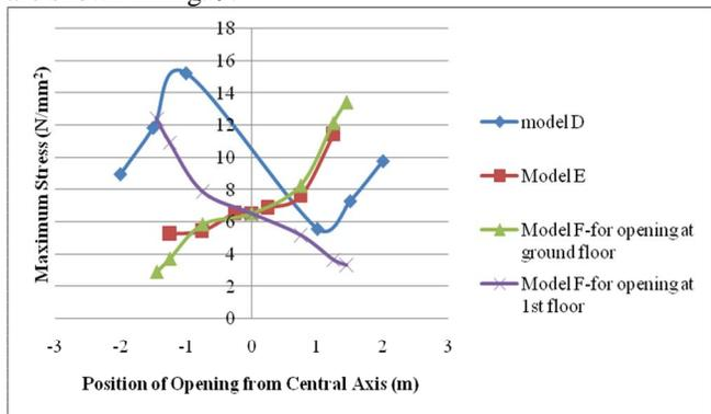
**Figure 9.** Percentage of Opening Vs Maximum Stress around Opening for Model D,E & F
