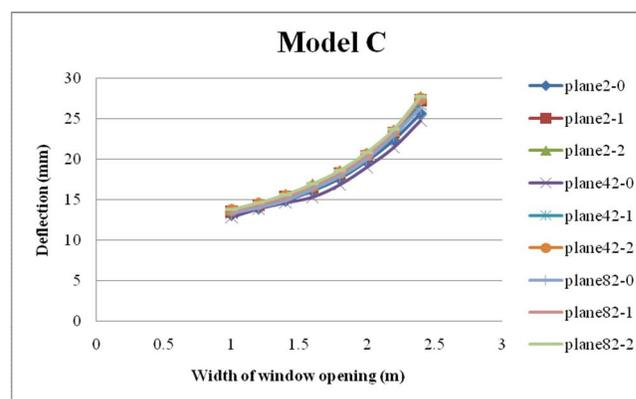
**Figure 4. Width of Opening Vs Deflection for Model C**
