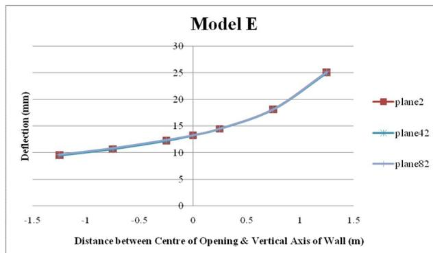
Figure 6. Position of Opening Vs Deflection for Model E
