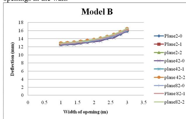
**Figure 3. Width of Opening Vs Deflection for Model B**
