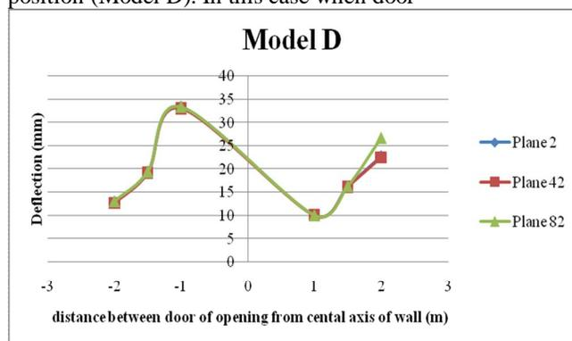
Figure 5. Position of Opening Vs Deflection for Model D
