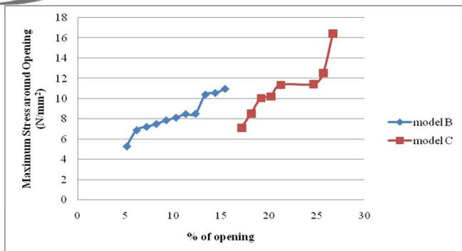
**Figure 8.** Percentage of Opening Vs Maximum Stress around Opening for Model B & C
