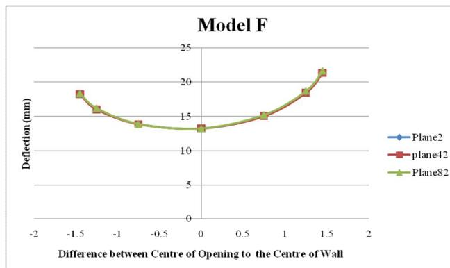
Figure 7. Position of Opening Vs Deflection for Model F
