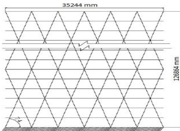
Figure 2. Typical Elevation of Diagrid Structure.
