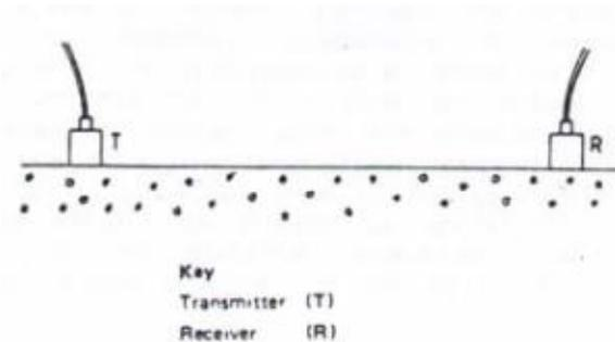
Fig.5(C): Indirect or surface transmission
