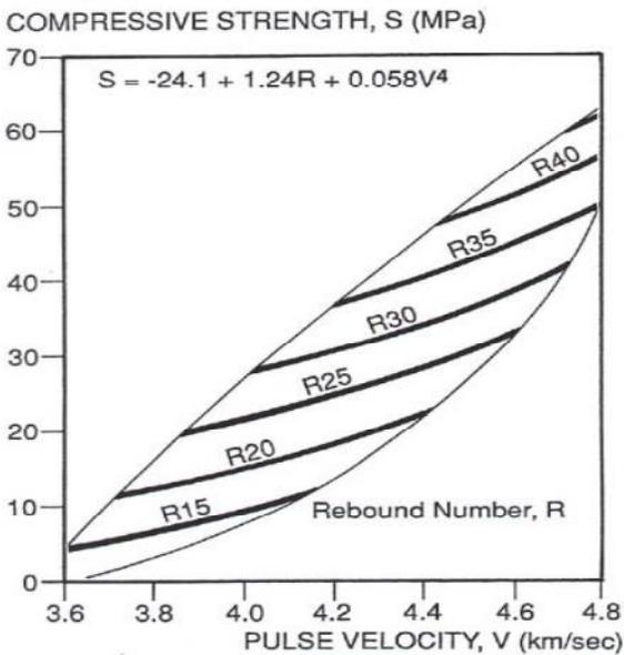
Fig.9 Nomogram for concrete of a particular aggregate type and age
