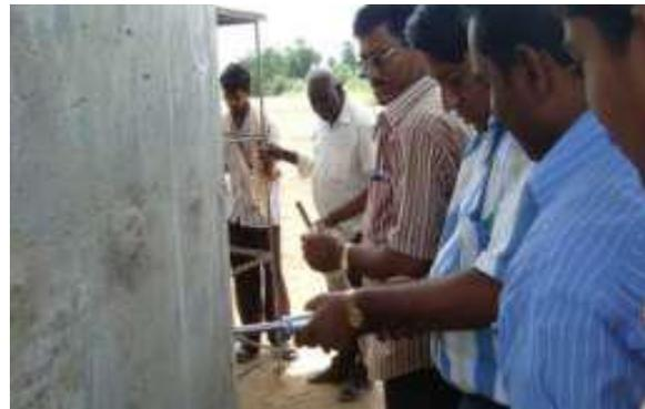
Fig.11 Testing of Bridge Pier using Rebound Hammer
