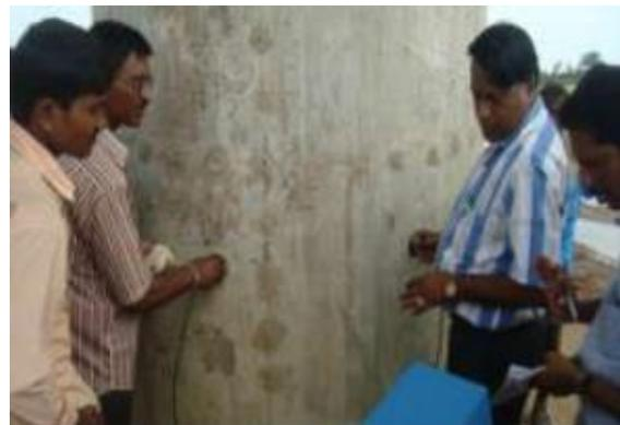
Fig.12 Testing of Bridge Pier using Ultrasonic Tester
