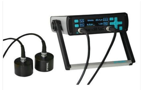
Fig 3. Ultrasonic pulse velocity testing instrument
