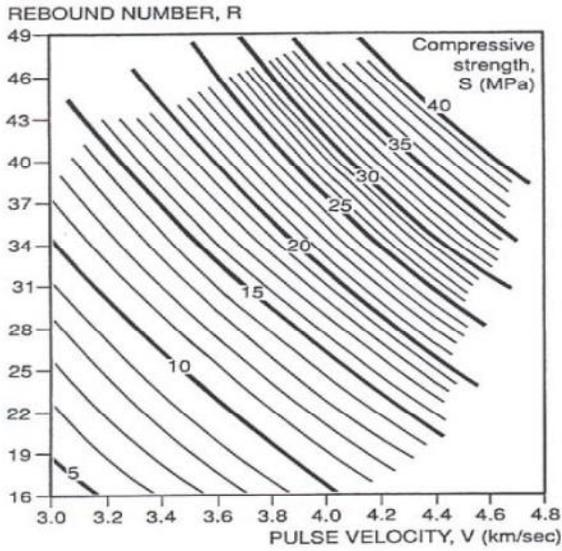
Fig.8 ISO-Strength curves concrete for reference in SONREB method
