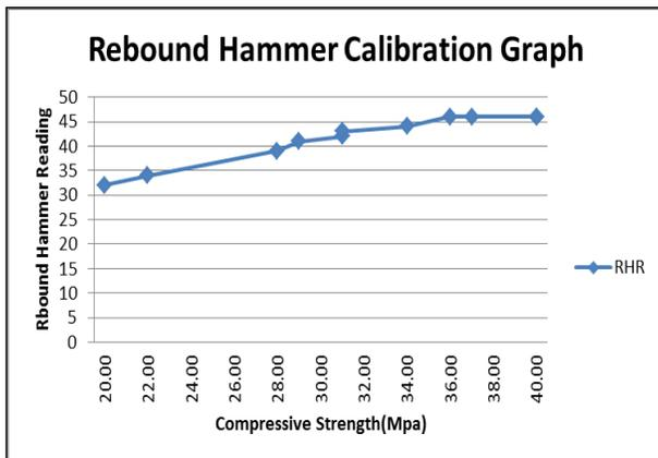
Fig2: Correlation between compressive strength of concrete and rebound hammer number
