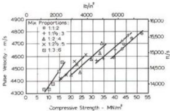
Fig.7. Relation between ultrasonic pulse velocity and compressive strength for concretes of different mix proportion
