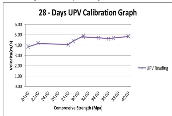
Fig.4 the calibration chart for compressive strength and ultrasonic pulse velocity
