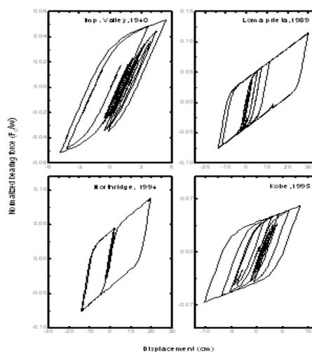
Fig. 8 Force-displacement hysteresis loops of R-FBI control for various earthquake ( $T_b=4s, \xi_b=0.1, \mu_b=0.04$ )
