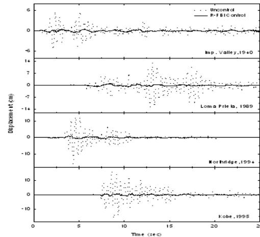
Fig. 5 Time varying displacement response of top floor ( $T_b = 4s, \xi_b = 0.1, \mu_b = 0.04$ )
