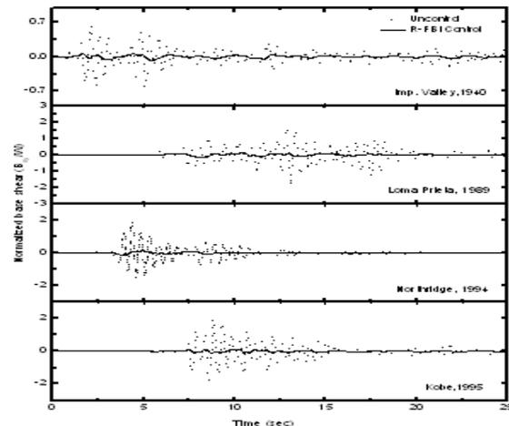
Fig. 7 Time variation of base shear responses ( $T_b = 4s, \xi_b = 0.1, \mu_b = 0.04$ )
