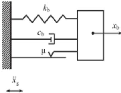
**Figure 4.** Schematic diagram of R-FBI system.
