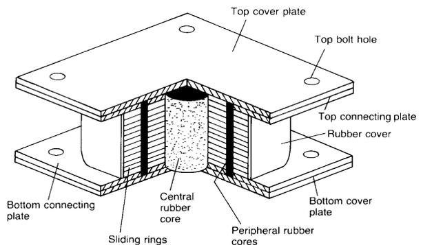
Figure 3. Cross section of R-FBI system.
