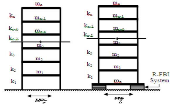
Figure 2. Structural model of Building with and without R-FBI system.
