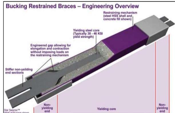
Figure 1. Buckling restrained brace.[2]
