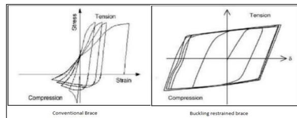
Figure 2. load tests on braces.[3]
