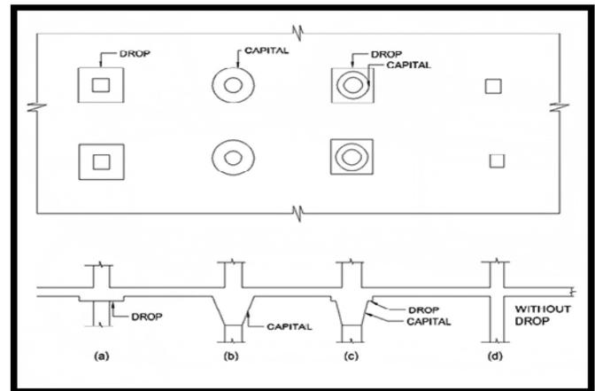
Figure 1 Types of flat slab
