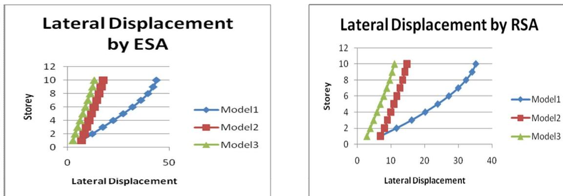
Figure 3. Lateral storey displacement by ESA and RSA
