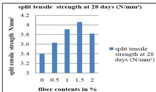
Figure 4: Variation of splitting tensile strength.
