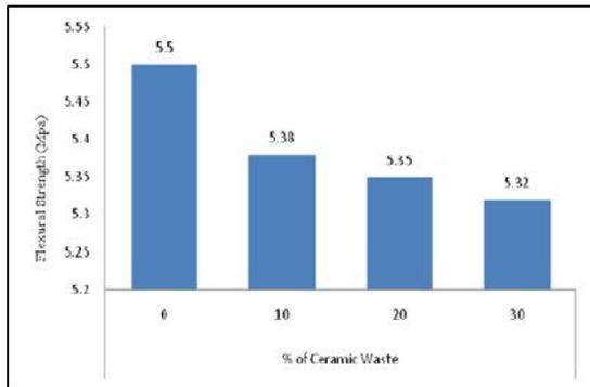
Figure 3: Variation of flexural strength.
