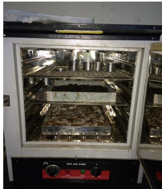
**Figure 3.** Heating Of Aggregate Samples
