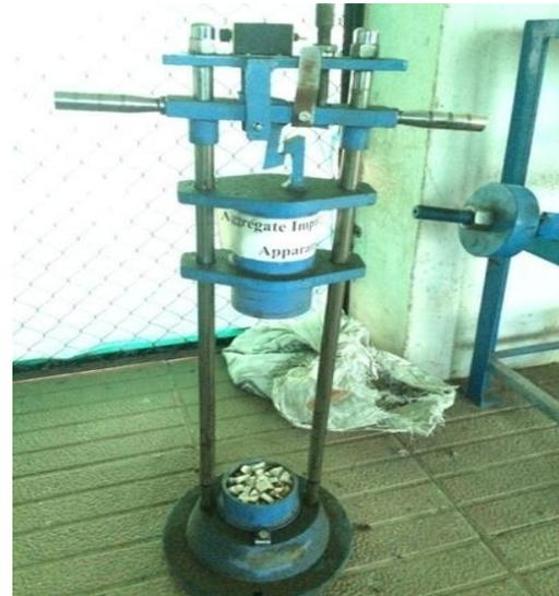
Figure 1. Impact Test
