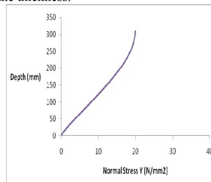
Figure 3. Variation of Normal stress (Y) through the thickness of composite beam
