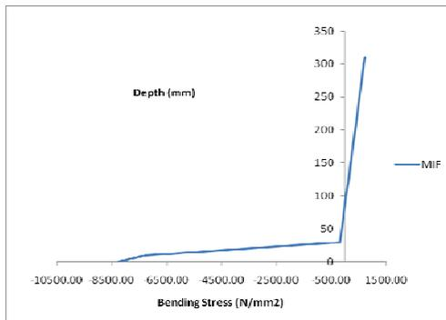
**Figure 5.** Variation of Bending stress ( $\sigma_x$ ) through the thickness of composite beam
