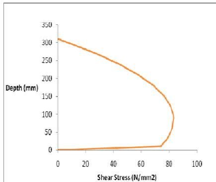
**Figure 4.** Variation of Shear stress (X) through the thickness of composite beam
