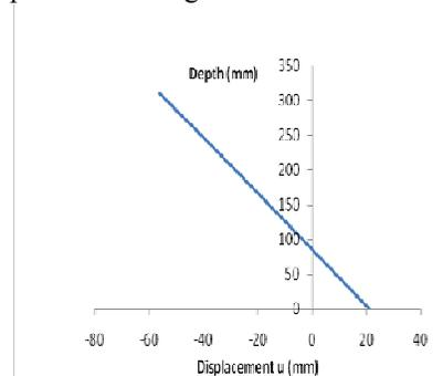
Figure 1. Variation of displacement (u) through the thickness of composite beam.
