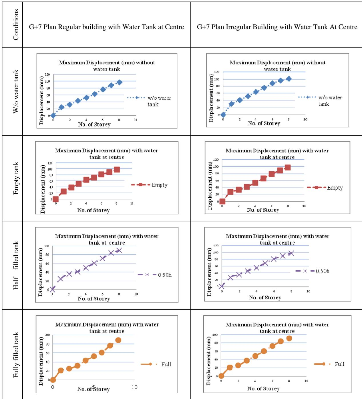
Figure 6. Details of displacement of G+7 plan regular and irregular building
