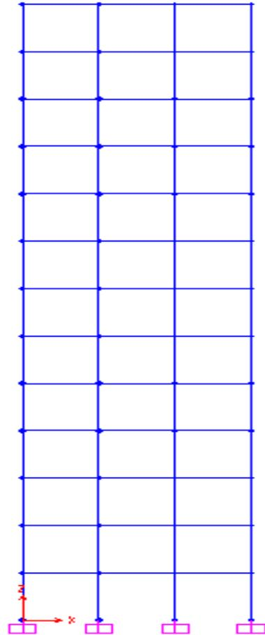
Figure 5. Elevation of G+12 storey building
