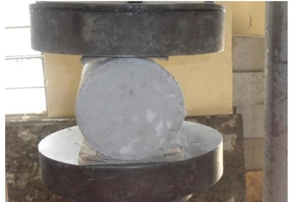
Figure 5. Split Tensile Test
