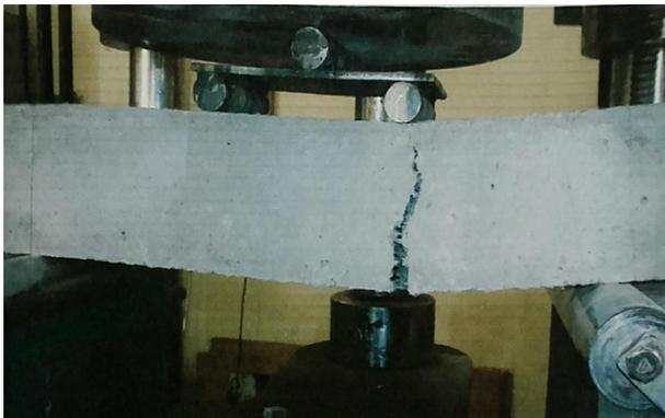
Figure4. Flexural behavior of Beam
