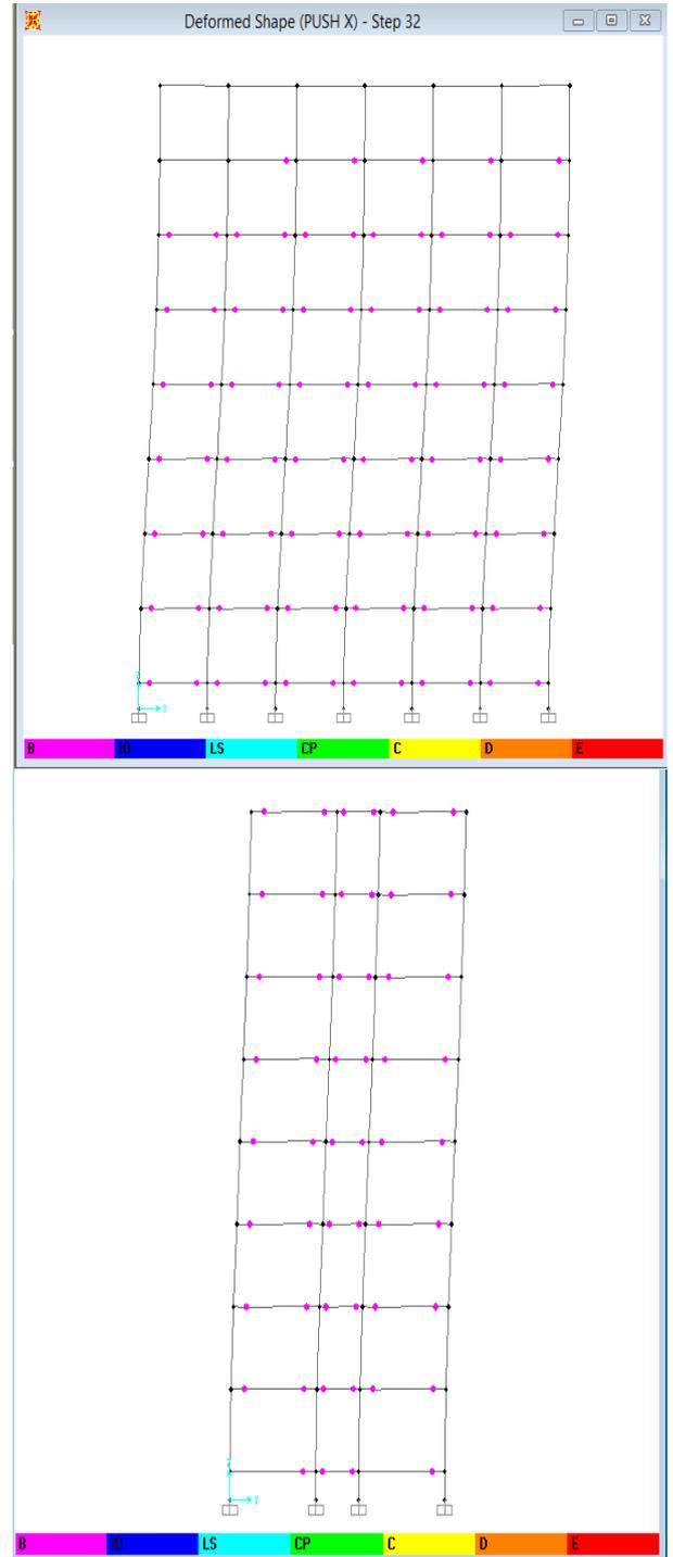
**Fig.10** Hinge formation at performance point for zone IV building without floating columns in X and Y direction
