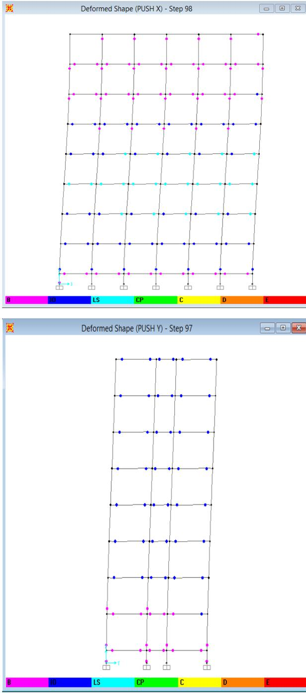
**Fig 11:** Hinge formation at performance point for zone V building without floating columns in X and Y direction
