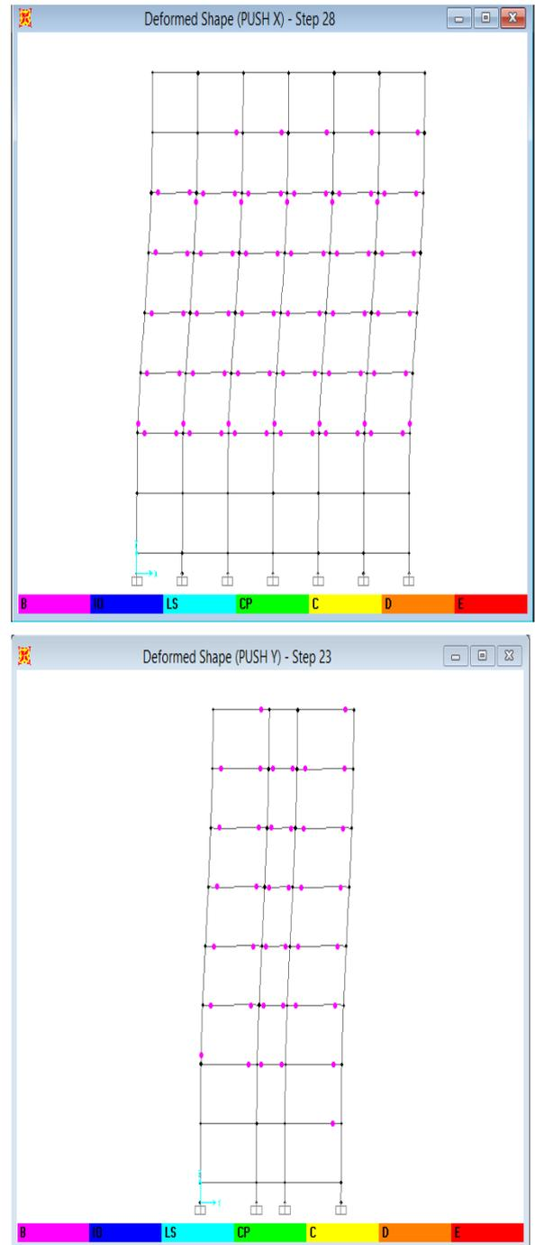
**Fig 16:** Hinge formation at performance point for zone IV building with floating columns in model III in X and Y direction.
