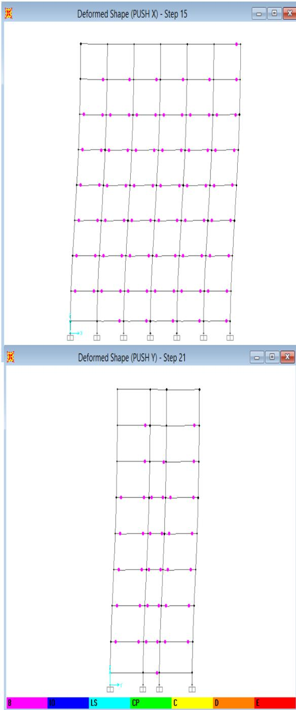
**Fig no 9:** Hinge formation at performance point for zone III building without floating columns in X and Y direction
