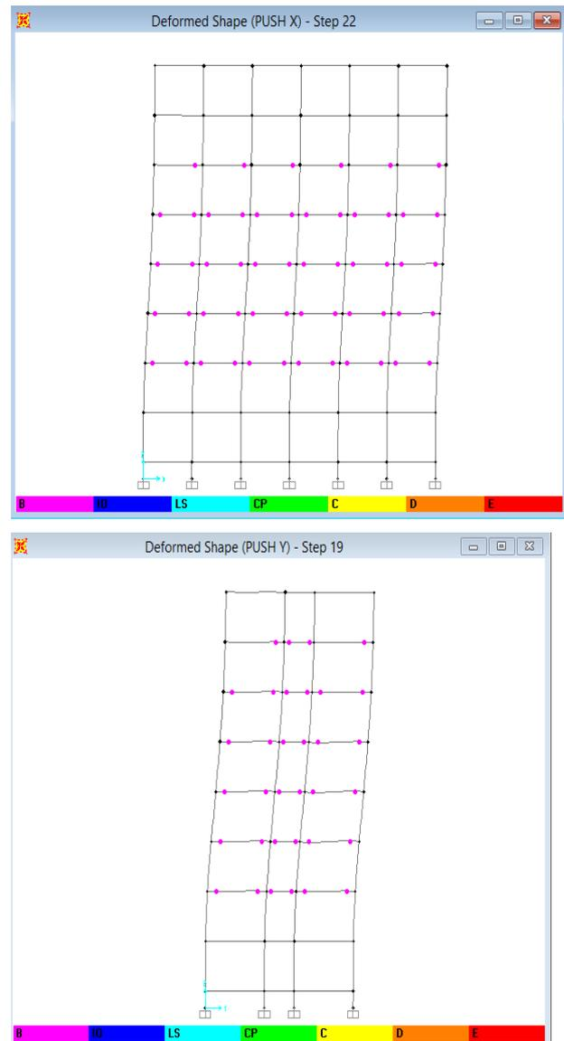
**Fig12:** Hinge formation at performance point for zone III building with floating columns in model II in X and Y direction
