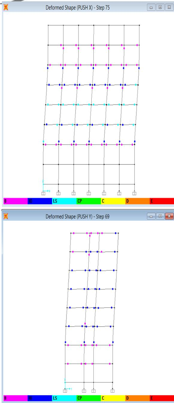
**Fig 17:** Hinge formation at performance point for zone 5 building with floating columns in model III X and Y direction
