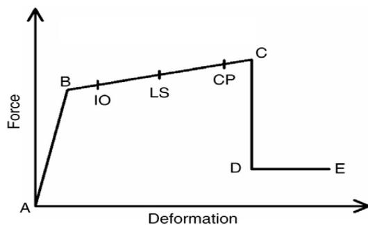
Fig 2. Force-Deformation for Pushover Hinge
