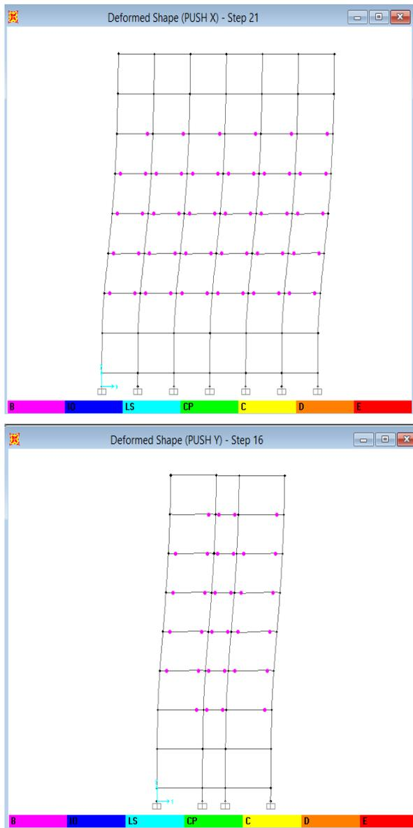
**Fig 15:** Hinge formation at performance point for zone III building with floating columns in model III in X and Y direction
