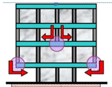
Figure 1 Fig.1 Floating columns building
