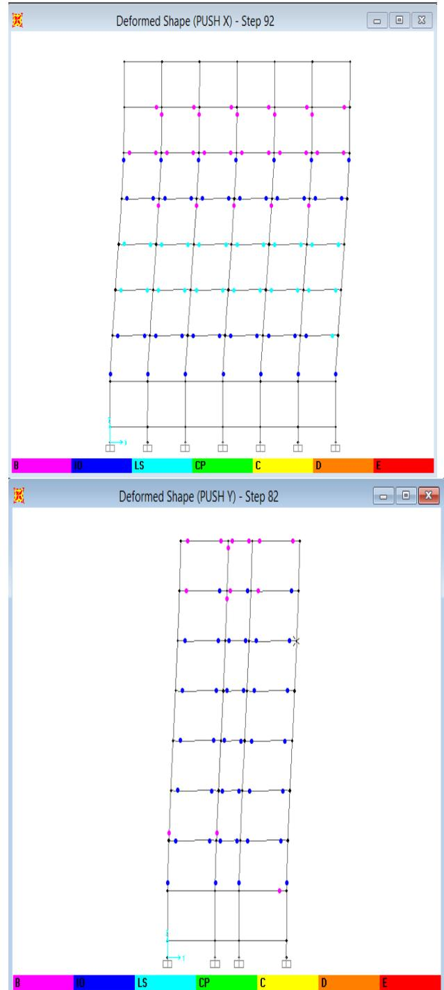
**Fig 13:** Hinge formation at performance point for zone IV building with floating columns in model II in X and Y direction
