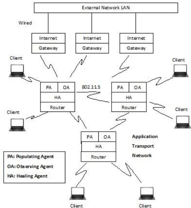
Fig. 1 Proposed overview model of scalable capabilities incorporated in Wireless Mesh Networks
