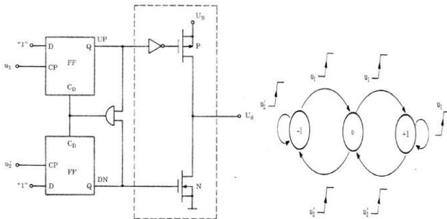
Fig. 2.3. Schematic diagram of the PFD and its state diagram. Phase frequency detector has two inputs that
