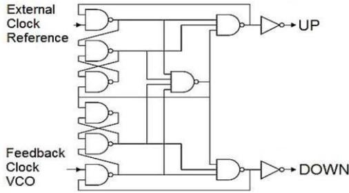
Fig 2.2 Conventional logic gates PFD
