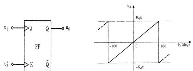
Fig. 2.1 Block diagram of JK flipflop phase detector and its characteristics.
