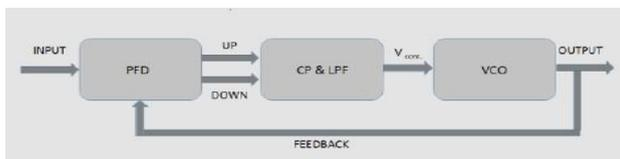
Fig. 1.1 Block diagram of Phase locked loop
