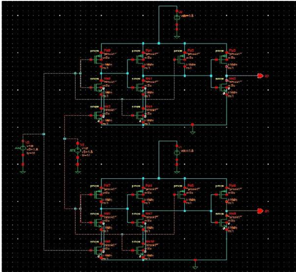
Fig 3.1.Design of phase frequency detector in cadence
