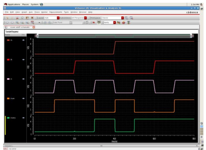
Fig.10. Transient response of 28T full adder
