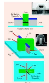
Fig 1: cross sectional view and plan view of FinFET
