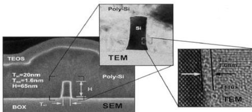
Fig 5: cross section of poly- si of FinFET
