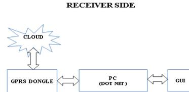
Figure.3 Block diagram of the receiver side
