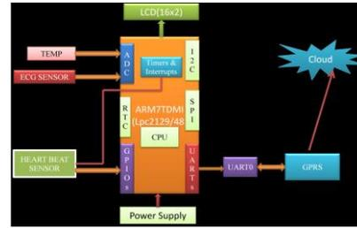
Figure.2 Block diagram of the sender side.
