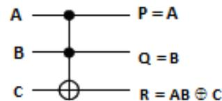
Fig.2.4: Circuit representation of Toffoli gate
