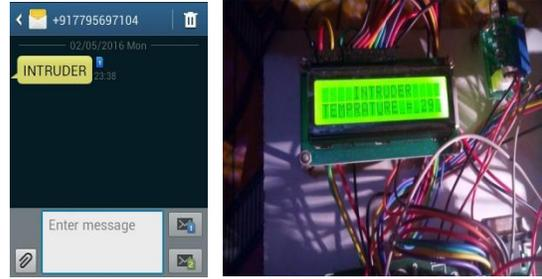
If the temperature of the transformer is going abnormal, the temperature sensor gets activated and the message “TEMPERATURE HIGH” is sent to the person at the maintenance department through the GSM module. The temperature value is displayed on LCD display.
