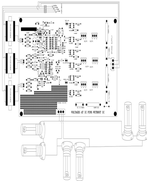
Fig: 6 The complete prototype and its circuit
