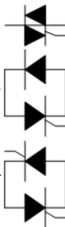
Fig: 2 Solid state switches
