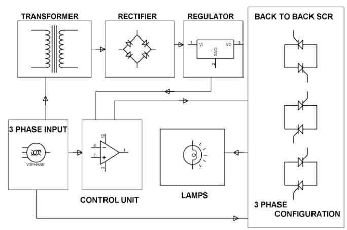
Fig: 1 Block diagram for soft starting of induction motor
