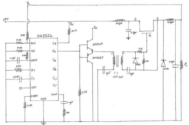
Fig.2: control circuit for buck converter
