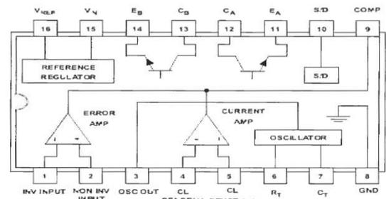
Fig.3: Pin diagram of SG3524
