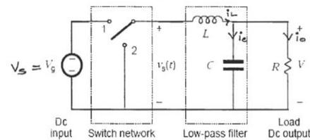
Fig1: Basic Circuit
