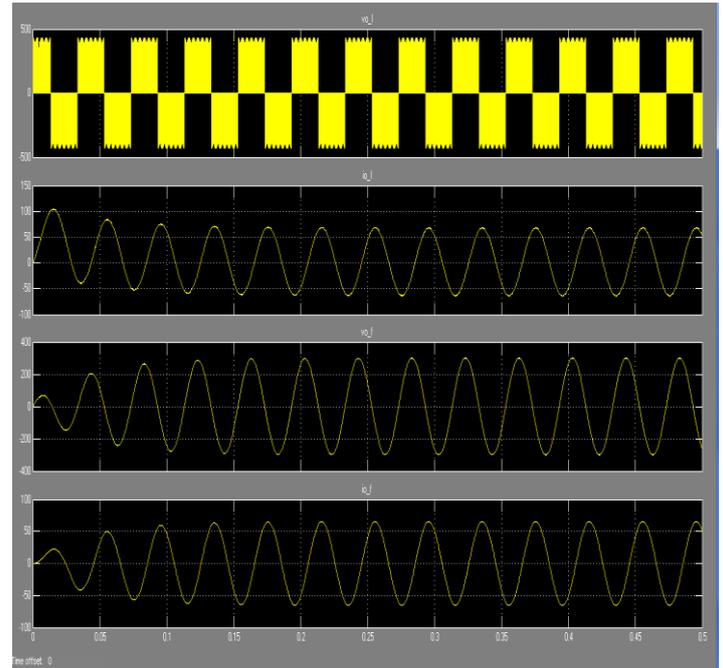
Figure 14: Captured waveform of output voltage, output line current, filtered output voltage and current for the filtered output line current for  $f_i = 50$  Hz and  $f_0 = 25$  Hz
