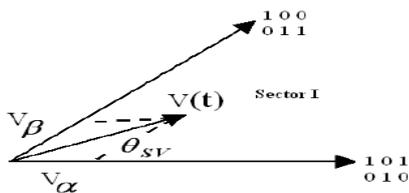
Figure.11. Vector Span of Voltage Space Vector in Sector 1
