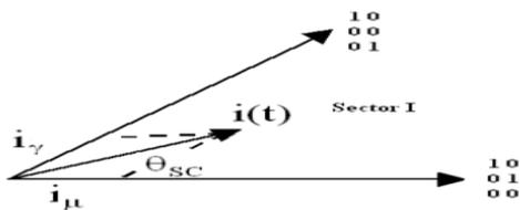
Figure.7. Vector span of current space vector in sector 1
