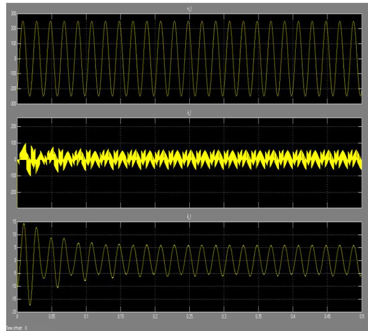
Figure 15. Captured waveform of input phase voltage, unfiltered input phase current and filtered input phase current for  $f_i = 50$  Hz and  $f_0 = 25$  Hz
