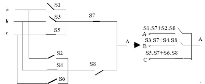
Figure.12. One phase VSI to one phase matrix converter
