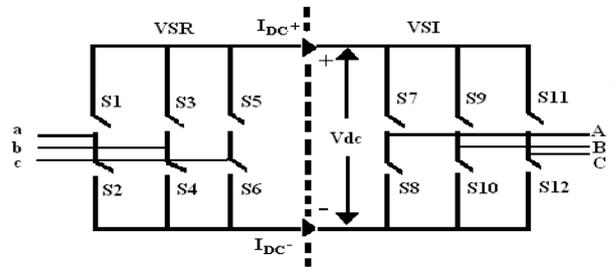
Figure.2. Equivalent circuit of 3x3 matrix converter
