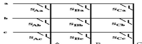
Figure 3: switch matrix of 3 phase MC
