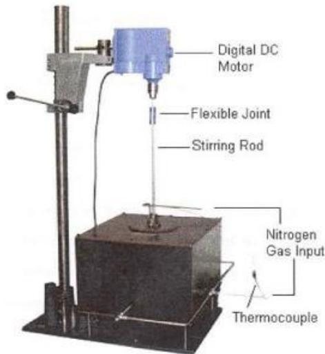
**Figure 1:** Stir casting setup
