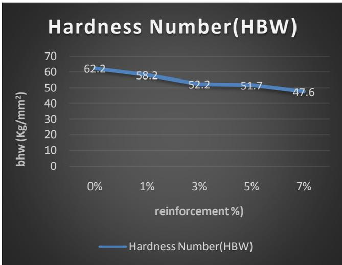
**Graph 1:** The BHN for Al Alloy 7075 reinforced with different wt. % of Al<sub>2</sub>O<sub>3</sub> material at room temperature.
