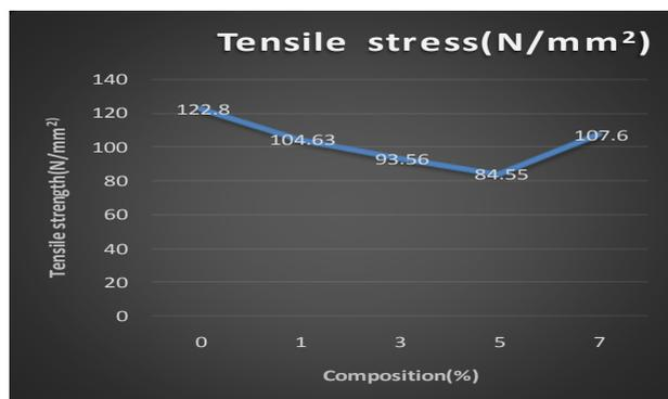
**Graph 2:** Shows the tensile strength vs composition % of Al<sub>2</sub>O<sub>3</sub>
