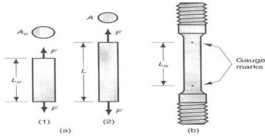
**Figure 4:** Tensile Test Specimen
