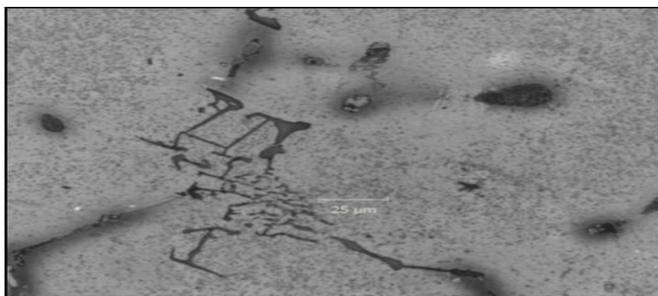
**Figure 6:** 500X With Keller's Reagent Al-Alloy 7075 Reinforced with 7% Al<sub>2</sub>O<sub>3</sub>
