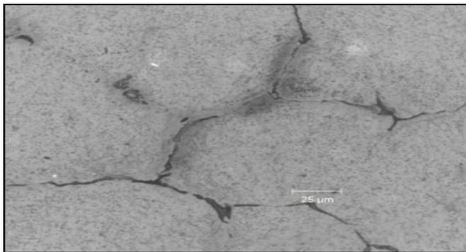
**Figure 5:** 500X With Keller's Reagent Al-Alloy 7075 Reinforced with 1% Al<sub>2</sub>O<sub>3</sub>
