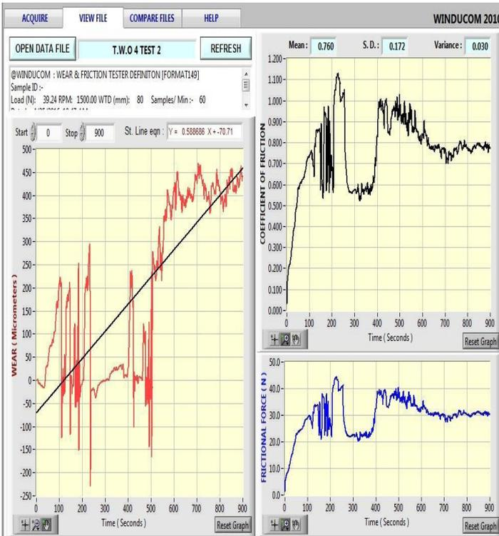
Graph 2: Wear, Coefficient of friction, Frictional force of PEEK 30% GLASSFILLED
