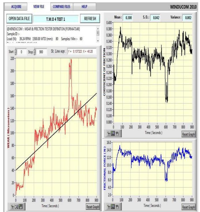
Graph 1: Wear, Coefficient of friction, Frictional force of PEEK
