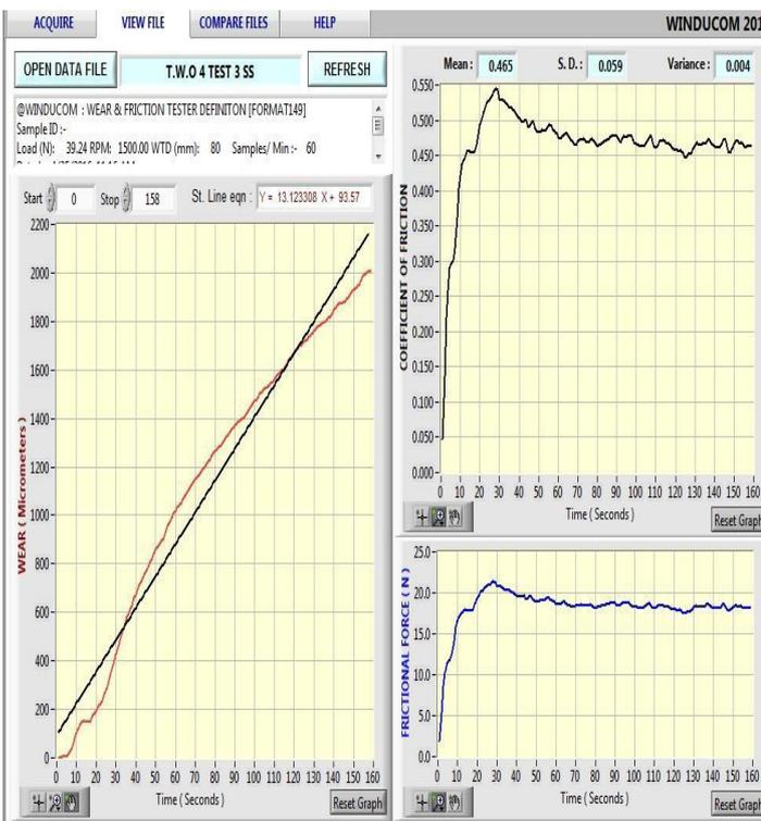
Graph 3: Wear, Coefficient of friction, Frictional force of SS304
