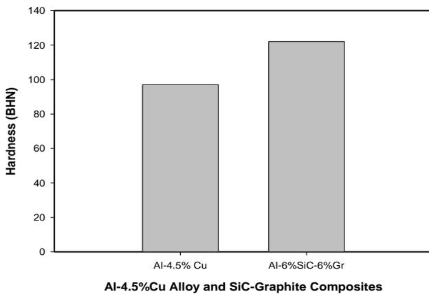
**Figure 3. Hardness of Al-4.5%Cu alloy and its composites**
