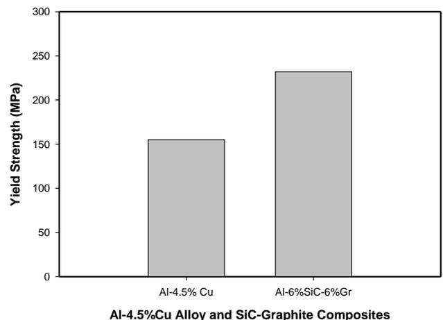
**Figure 5. Yield strength of Al-4.5%Cu alloy and its composites**
