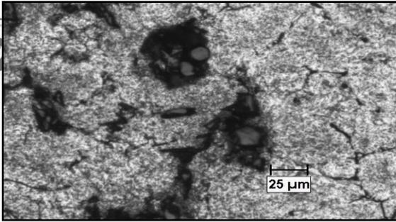
**Figure 2. Optical micrographs of (a) as cast Al-4.5Cu alloy (b) Al-4.5% Cu-6 wt. % SiC & 6 wt. % Graphite composites**
