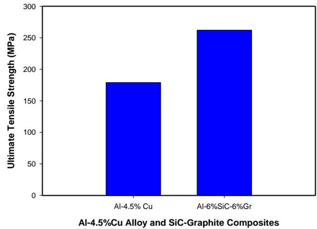
**Figure 4. Ultimate tensile strength of Al-4.5%Cu alloy and its composites**
