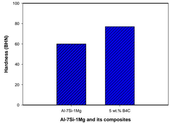
Fig.2: Variation of Al-7Si-1Mg with 5wt. % of B<sub>4</sub>C particulates in Hardness before and after addition
