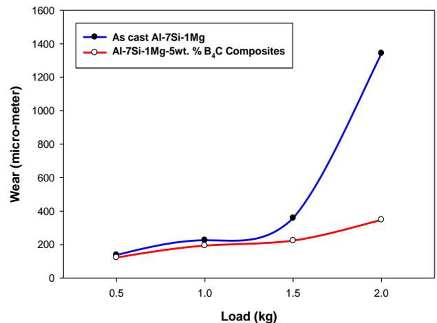
Fig.3: Showing wear in height loss of as cast Al-7Si-1Mg and its composites at varying loads
