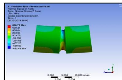
Fig. 10: Normal Fiber Stress in the  $Fe_{2-3}N$  Layer in Composite Layer of Thicknesses of  $T(Fe_4N) = 10 \mu m + T(Fe_{2-3}N) = 10 \mu m$
