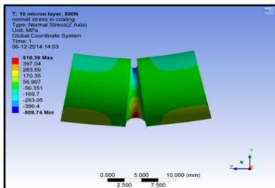
Fig. 7: Normal Fiber Stress in the Untreated Specimen
