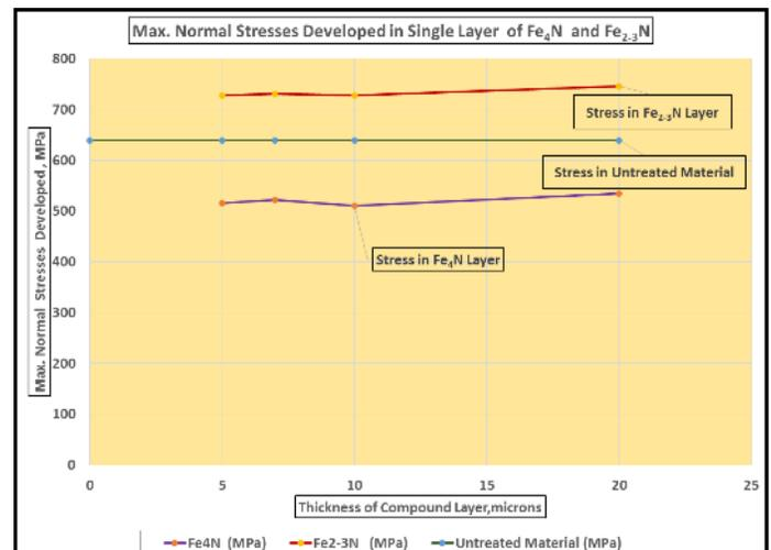
Fig. 11: Maximum Normal Fiber Stress in the Untreated Specimen and single layers of  $Fe_4N$  and  $Fe_{2-3}N$
