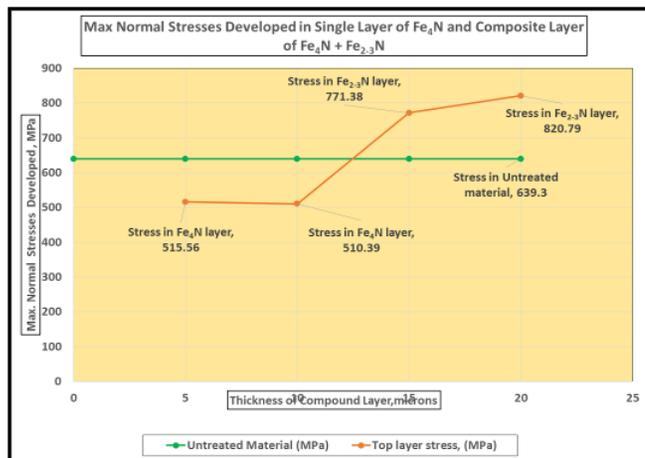
Fig. 12: Maximum Normal Fiber Stress in the Untreated Specimen, single layer of Fe<sub>4</sub>N layer & composite layer of Fe<sub>4</sub>N+Fe<sub>2-3</sub>N
