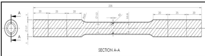
Fig. 1: Schematic of the fatigue test specimen
