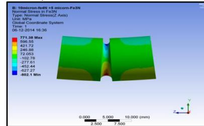
Fig. 9: Normal Fiber Stress in the  $Fe_{2-3}N$  Layer of Composite White Layer of Thicknesses of  $T(Fe_4N) = 10 \mu m$  &  $T(Fe_{2-3}N) = 5 \mu m$
