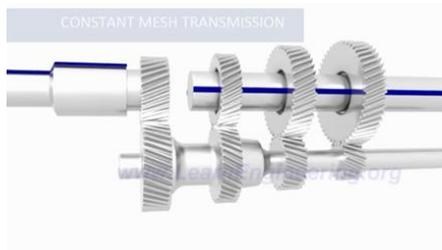
Fig. 1: Constant Mesh Transmission
