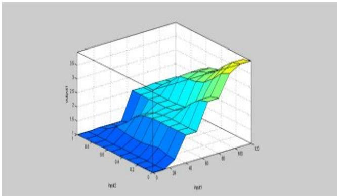
**Fig. 9:** The 3D surface view for the gear indication system using the surface viewer tool. The FIS input variables 'speed' and 'load' are plotted on the x and y axes respectively and the FIS output variable 'gear' is plotted on the z axis
