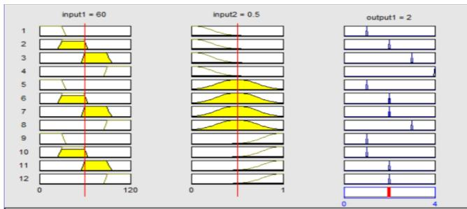
**Fig. 8:** The rule view for sample FIS input values 60 and 0.5 of speed and load respectively, generating the FIS output value 2 for optimal gear selection
