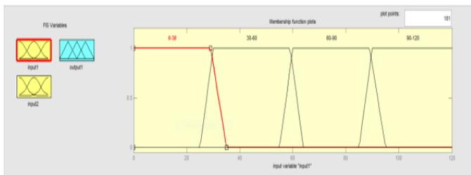
**Fig. 4:** Membership function plot for the first FIS input variable ‘speed’
