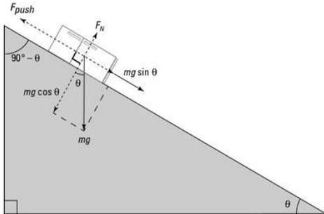
**Fig. 3:** Free body diagram of a vehicle moving up on an inclined road
