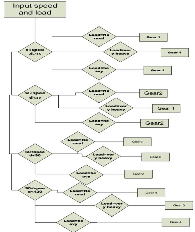
**Fig. 6:** Block diagram of the gear indication system
