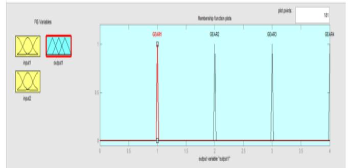
**Fig. 7:** Membership function plot for the FIS output variable ‘gear’
