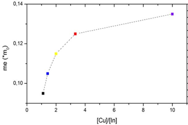
**Figure 2:** Variation of the effective masse of electron ( $m_e$ ) according to ratio  $\frac{[Cu]}{[In]}$
