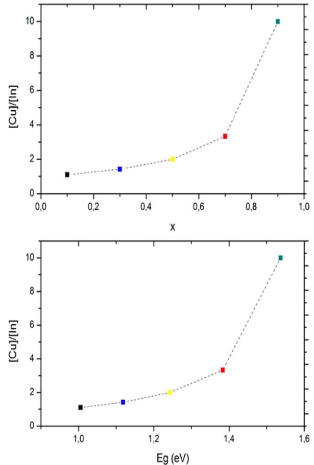
**Figure 1:** Variation of  $\frac{[Cu]}{[In]}$  ratio according to x (a) and the bandgap  $E_g$  (b).
