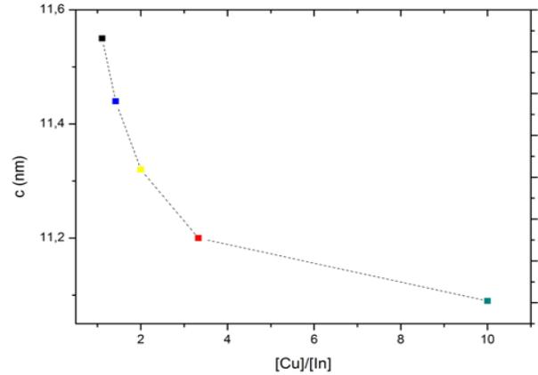
**Figure 3:** Evolution of the lattice parameter according to ratio  $\frac{[Cu]}{[In]}$ . (y) a ;(w) b
