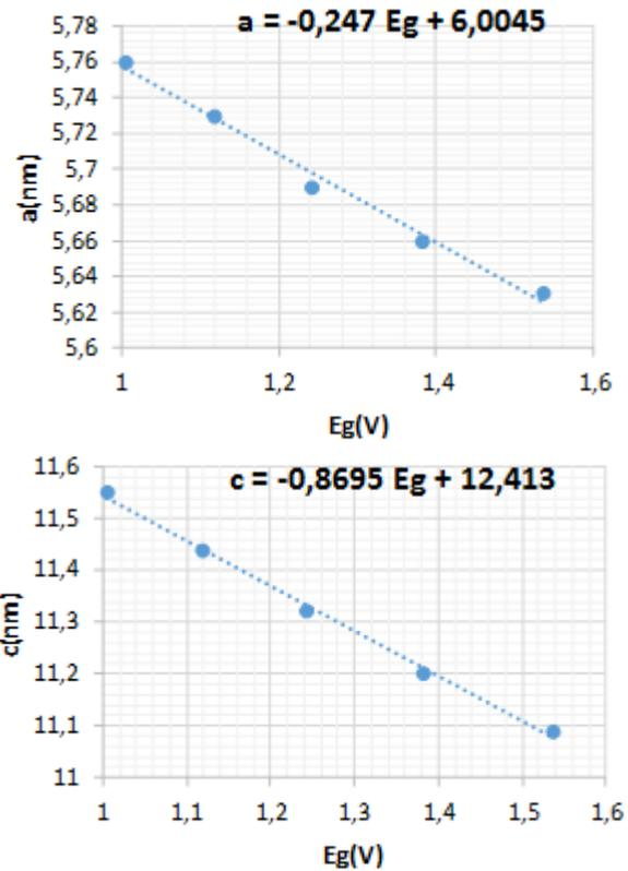
**Figure 5:** Variation of the lattice parameters  $a$  and  $c$  according to the bandgap  $E_g$
