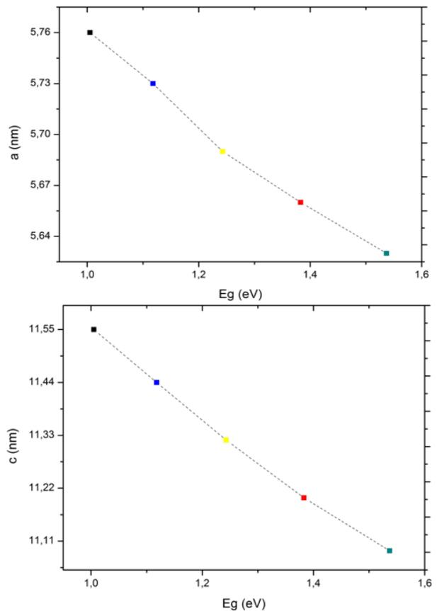
**Figure 4:** Lattice Parameters (a; c) according to bandgap  $E_g$ . We note a linear regression of the crystal parameters according to the bandgap. Here mathematical relations can be
