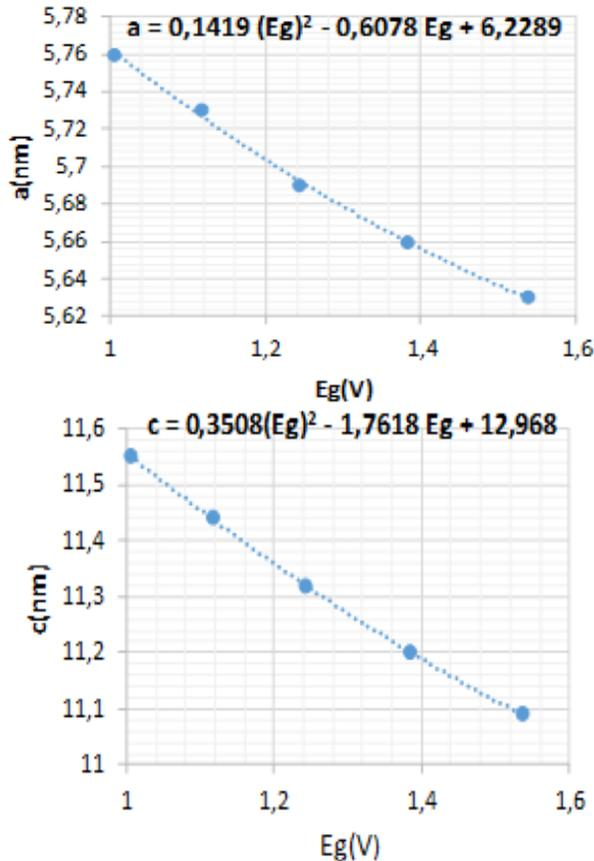
**Figure 6:** Variation of lattice parameters a and c according to  $E_g$ .
