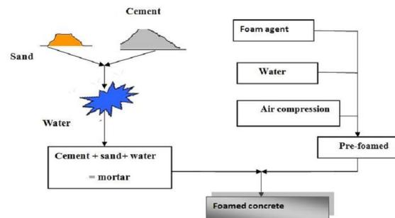
Figure 2 Manufacturing Process of Foamed Concrete
