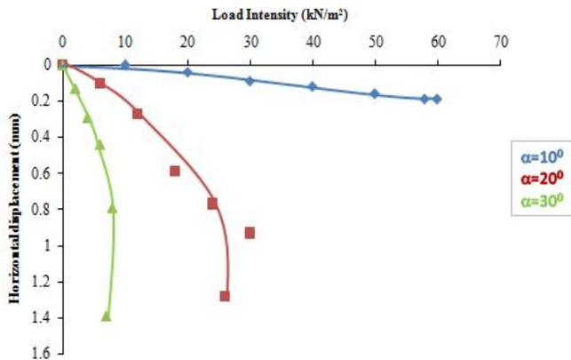
Figure 5: Horizontal Displacement vs. Load Intensity for Footing under Eccentric-Inclined Load at e/B=0.1.
