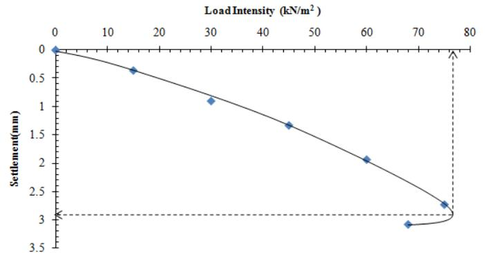
Figure 3: Load-Settlement Curve for Footing under Eccentric Load ( $e/B=0.1$ )
