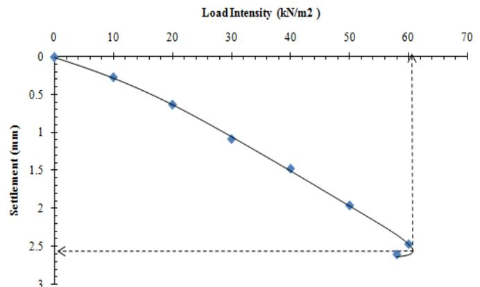
Figure 4: Load-Settlement Curve for Footing under Eccentric-Inclined Load ( $e/B=0.1$  and  $\alpha=10^0$ )
