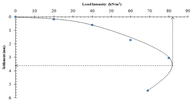
Figure 2: Load-Settlement Curve for Footing under Inclined Load ( $\alpha=10^0$ )
