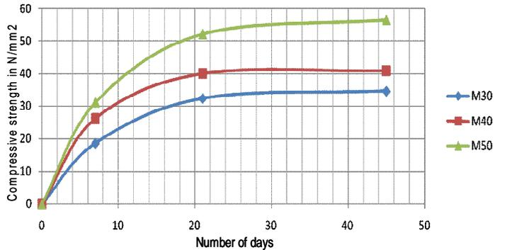
Figure 5: 40 % Fly Ash Replaced
