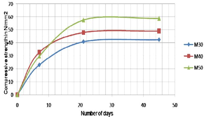
Figure 4: 30 % Fly Ash Replaced
