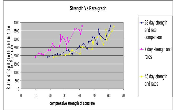
Figure 8: Compressive Strength Vs Rate of Concrete.
