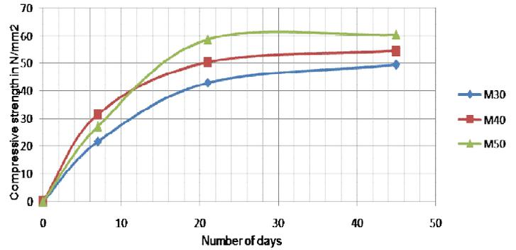
Figure 3: 20 % Fly Ash Replaced
