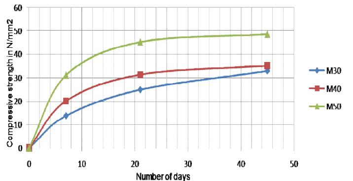
Figure 6: 50 % Fly Ash Replaced
