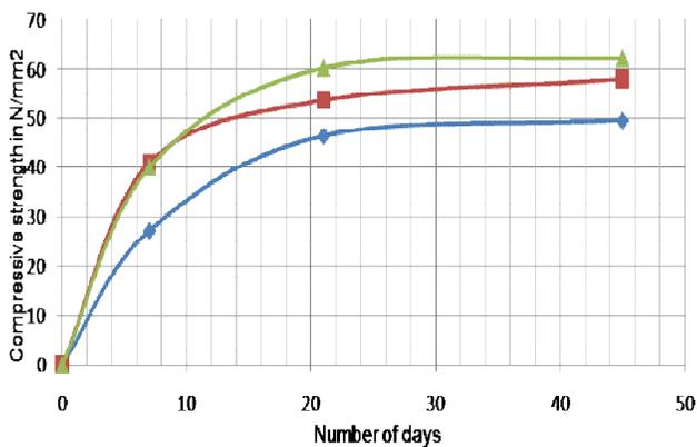
Figure 2: 10 % Fly Ash Replaced
