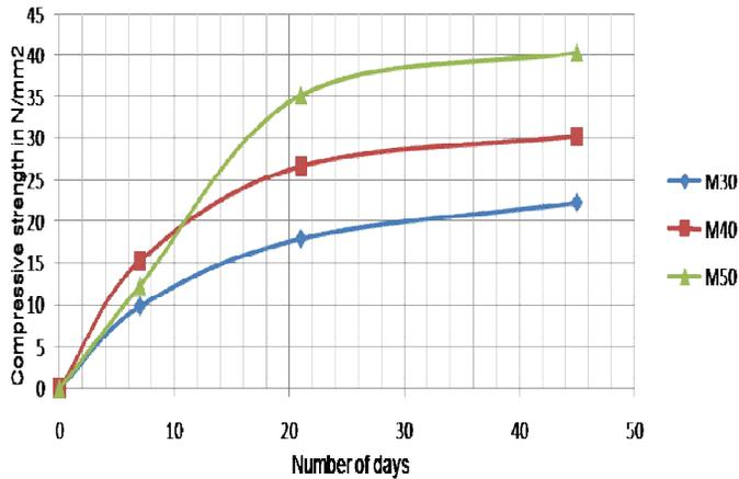
Figure 7: 60 % Fly Ash Replaced
