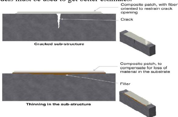
Fig. 2. Concept of the composite repair for cracks and corrosion thinning in metal substrates of FOU.
