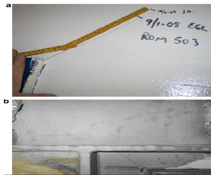
Fig. 3. Location and state of the fatigue crack in the Norne FPSO that was used as Demonstrator 1. (a) Crack as seen from the corridor side of the bulkhead. (b) Crack as seen from inside the room.
