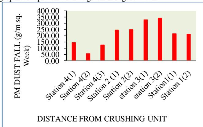
Fig2. PM dust fall ( $g/m sq. Week$ ) vs distance from crushing unit
