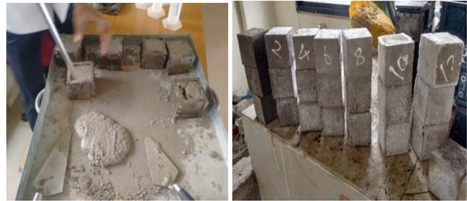
Image 2: Casting and Curing of Geopolymer Mortar
