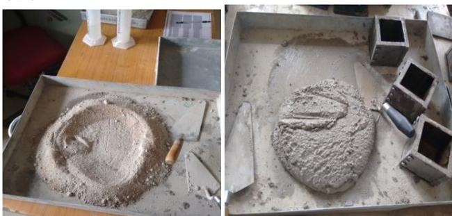
Image 1: Dry mixture and paste of Geopolymer Mortar
