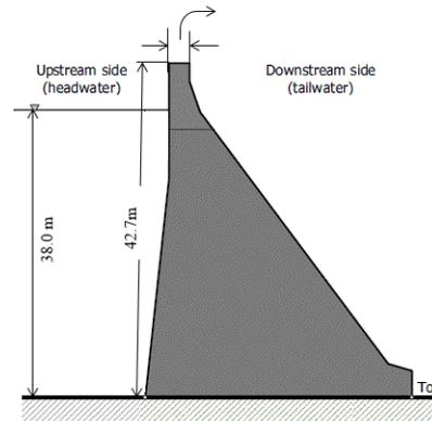
Figure 2: Section of Breach
