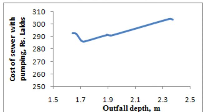
**Fig. 4:** Cost of pumping sewer vs outfall depth
