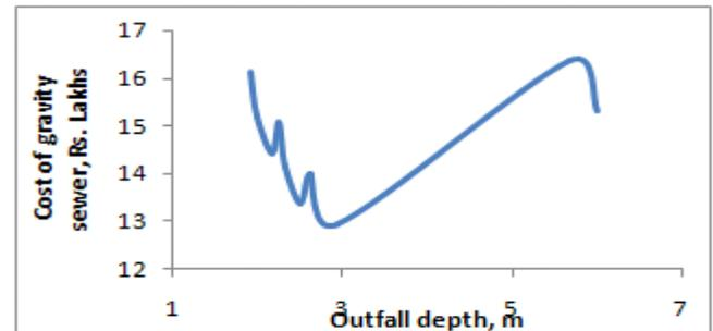
**Fig. 2:** Cost of gravity sewer vs outfall depth
