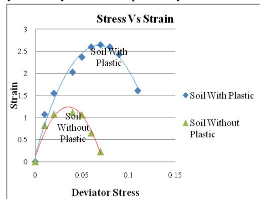
**Figure 2** Deviator stress versus strain while performing Tri-axial test
