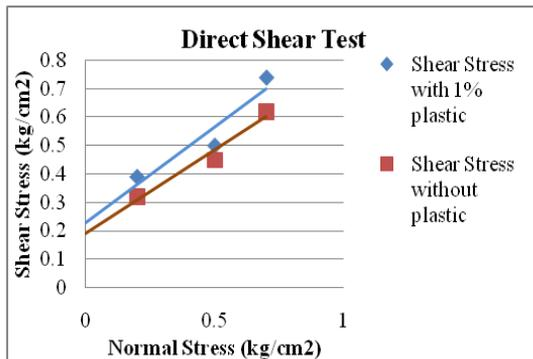
**Figure 3** Direct shear test results comparison
