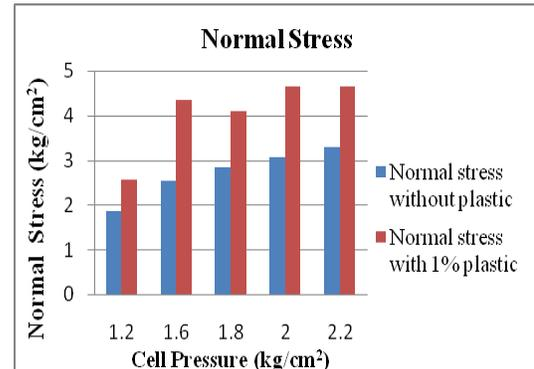
**Figure 1** Comparison of normal stress at same cell pressure Similarly Fig. 2 shows increase in strain and stress carrying capacity of soil by addition of plastic by 1%.
