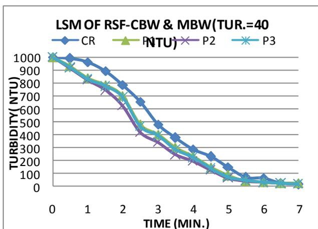
Figure 3 Ripening of Rapid sand filters:
